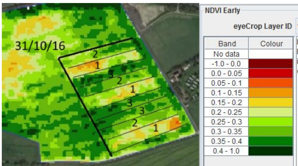
Figure 4-1 Satellite (NDVI) imagery of the trial area in October 2016; NDVI of 1.0 (dark green) indicates full crop cover; NDVI of 0 (red) indicates bare soil.
